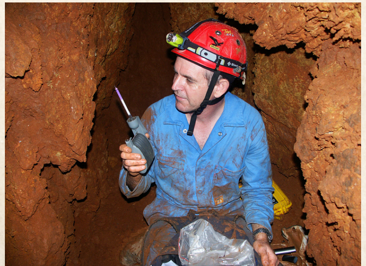
Fig. 5. Garry Smith using a Dräger meter to measure the CO 2 concentration in Doug Cave (GR9)
