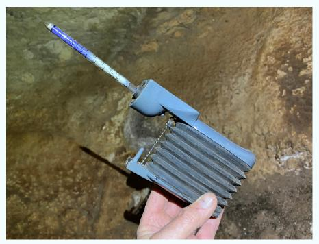
Fig 4 Dräger-Tube gas analyser is showing by the change in tube colour to purple, that there is a 4% CO2 concentration in Moores Cave, Timor, NSW
