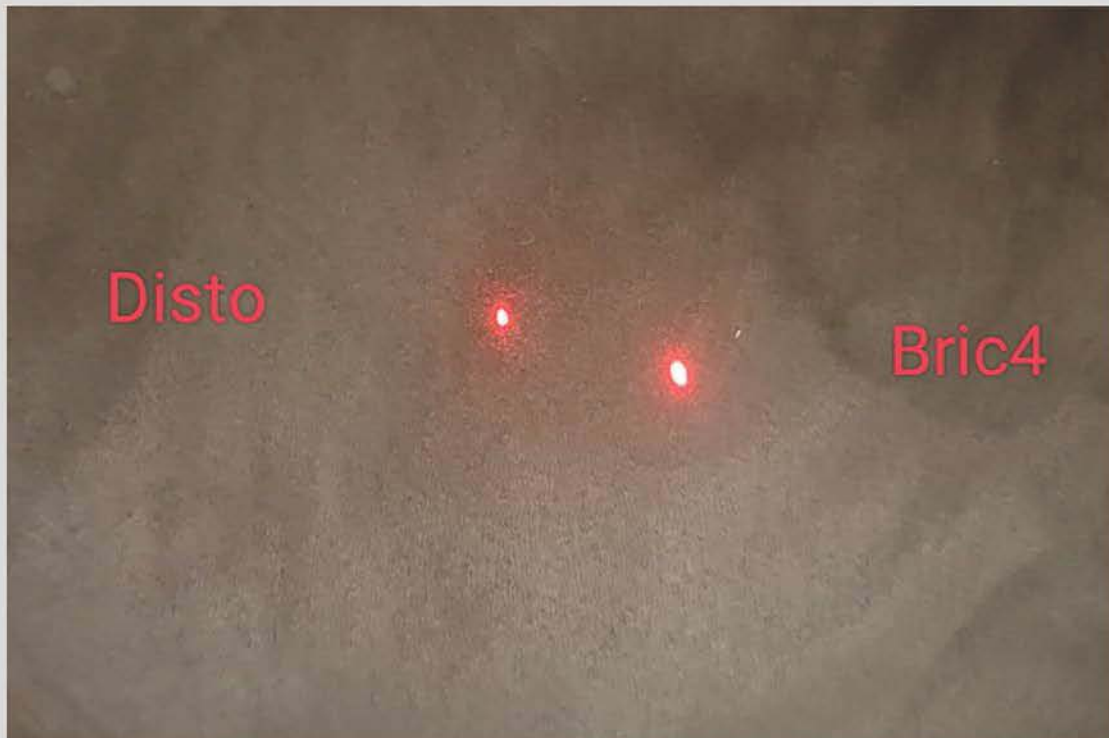
Photo by Bogdan Muresan Size comparison for laser point from 2 m distance
