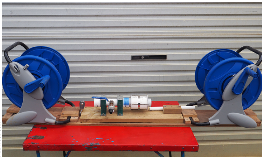
Two plastic hose reels make an easy-to-use rope washer
