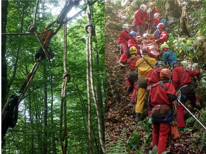
Photo above on the left - Using a Basic as progress capture on the haul for a Tyrolean seemed a default technique.
