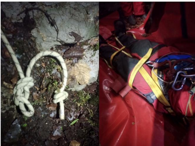
Photo above on the left - All haul lines are marked like this. A figure 8 and barrel knot for stopper. Not the fusion knot as the marker.
