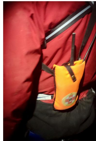
Photo above - UHF radios were carried by all the instructor/assessor team (it was a big, open shaft and cave). They were protected inside these simple, relatively waterproof and padded, pouches.
