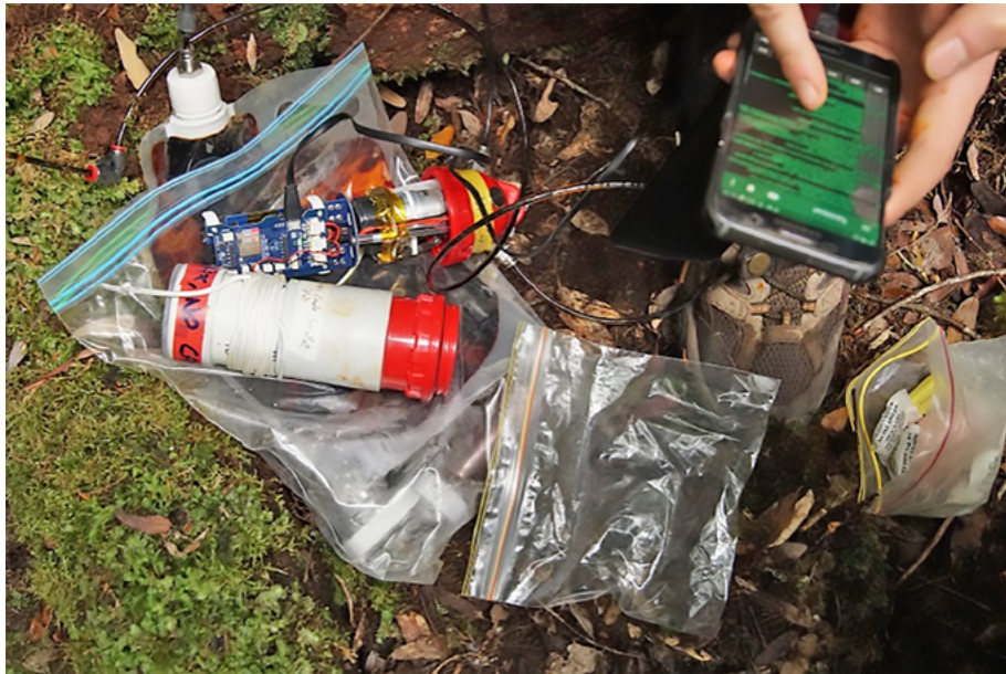
Reconfiguring a dye dispenser in the field
