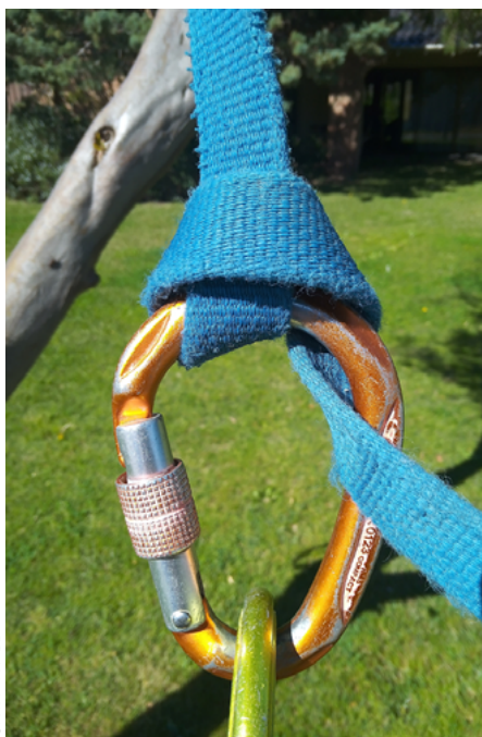
Figure 7: A Munter works OK on tube tape of 25 mm or thereabouts. It's probably not good for the tape. If you potentially have a freehanging, heavy buddy, use a SuperMunter knot. (Look it up)
