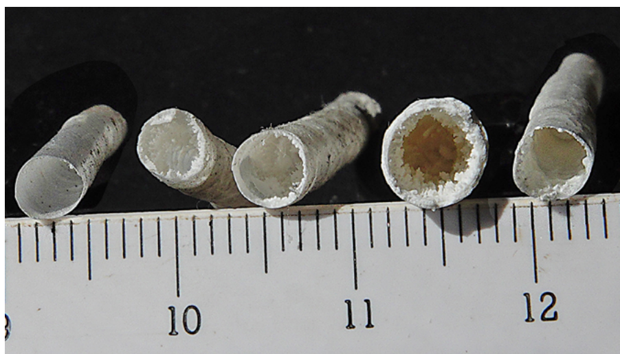
Figure 2: Typical cross-sections of calthemite straws. These have a thinner wall, are more fragile and have a less dense crystal structure than do speleothem straws. The image scale divisions are in mm.
