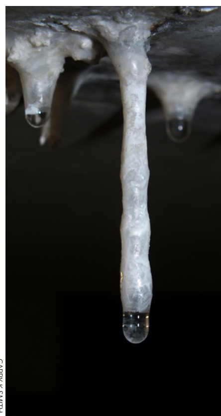
Figure 8: Variations in calthemite straw diameter, due to changes in solution surface tension, influenced by solution saturation of \text{Ca}(\text{OH})_2 and usually associated with changes in solution supply (drip rate).
