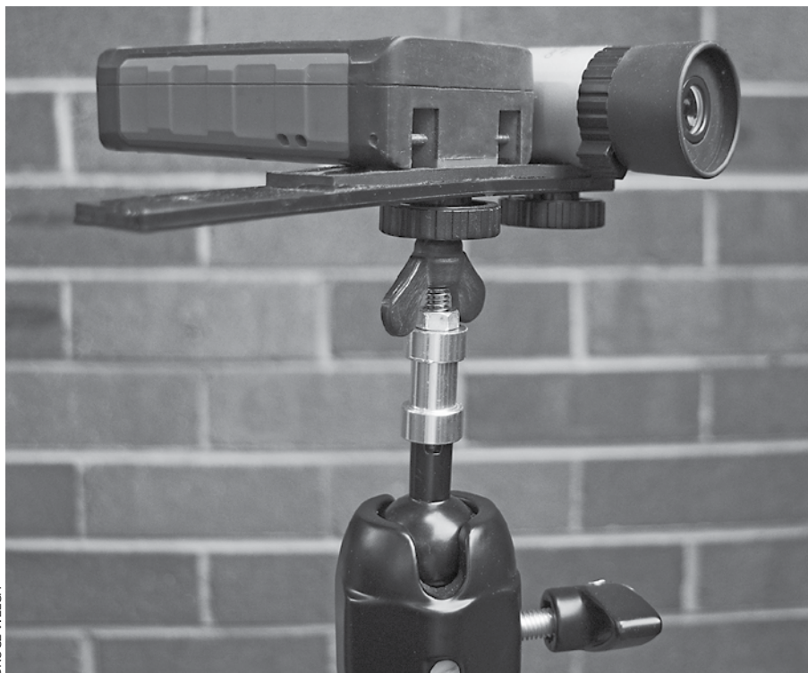
Disto/Monocular combo (connectors above the ball have since been reduced to approximately 10mm)
