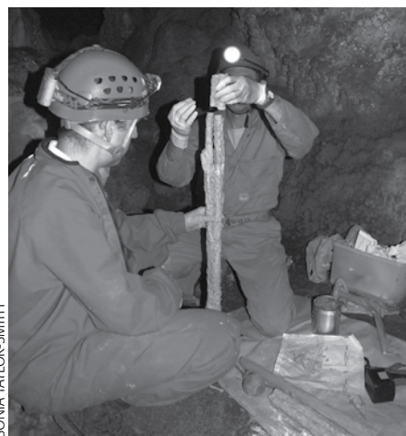
Checking the alignment before inserting pins and glueing
