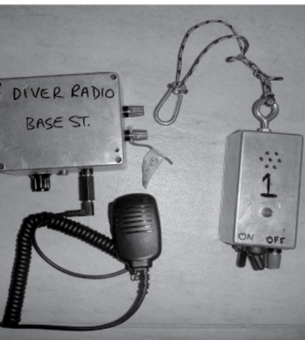
The cave radio system built for the habitat. by Joe Sydney
