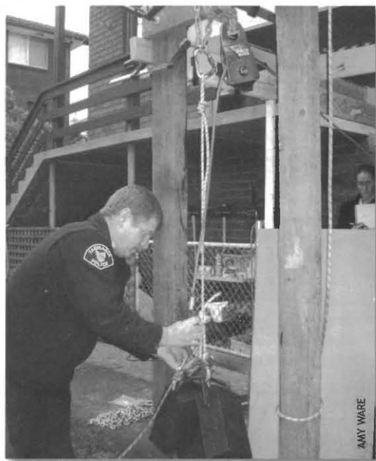
Damian Bidgood reattaching the winch cable to the test weight.
