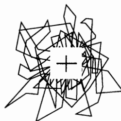
Figure 1 Typical track plot when GPS is at a fixed location. The centre of the plot is the average position.
